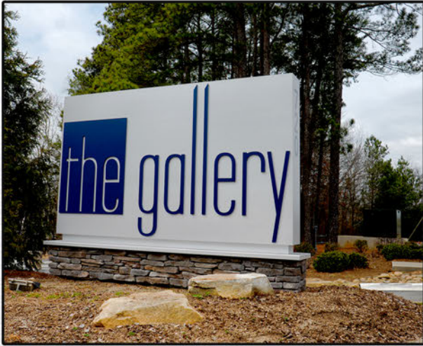
1/2" ALUMINUM PANEL with ROUTED COPY MOUNTED FLUSH TO CABINET PAINTED TO MATCH PMS 2956C (BLUE) (WHITE COPY IS CABINET BEHIND PANEL)
