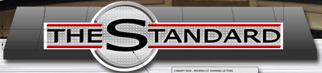
CANOPI SIGN - REVERSE LIT CHANNEL LETTERS BLACK FACES & RETURNS PERFORATED BRUSHED ALUMINUM MOUNTING PLATE WHITE ALUMINUM BACKER TO HIDE RACEWAYS
